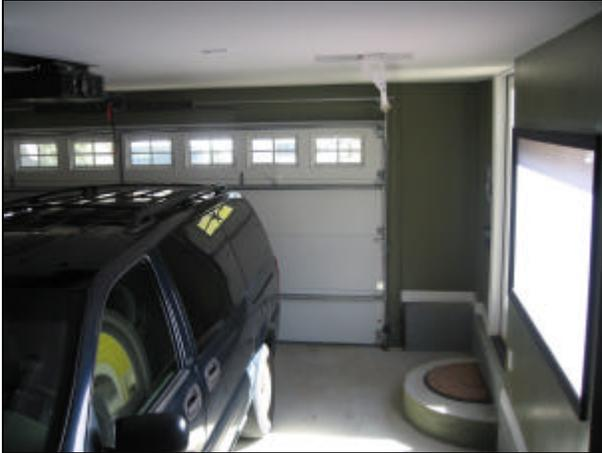
Installing a screen in this type of application is as simple as designing a window opening in a new home or adding a window in an existing home and actually proves to have many advantages. The screen location allows for the projector and any other components to be safely installed inside the garage where they are protected from the weather. In this case, US Nippura suspended the projector from the ceiling and connected it to the components in the projector room with
