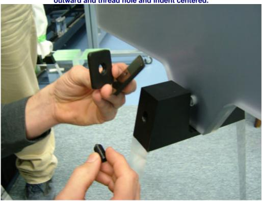
Step 1: Holding sandwiched with forefinger and thumb, slide in from the side between flange and stand, do not try to slide in from the top as you may scratch the screen surface/coating.
