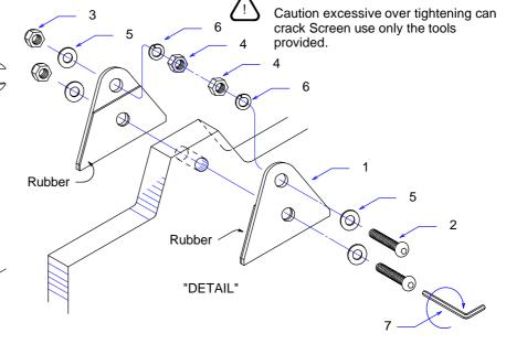
Attach suspension cable system following safety and engineering criteria of applicable Local Codes threading connectors/cables (not provided by manufacturer) between screen flange and top button bolt. Suspend with cables straight up and down ONLY. Do not attempt to suspend Screen at forced angles. Periodically check to make sure all components of asssembly are tight. Remove remaining clear protective film and store for future use and repacking.
