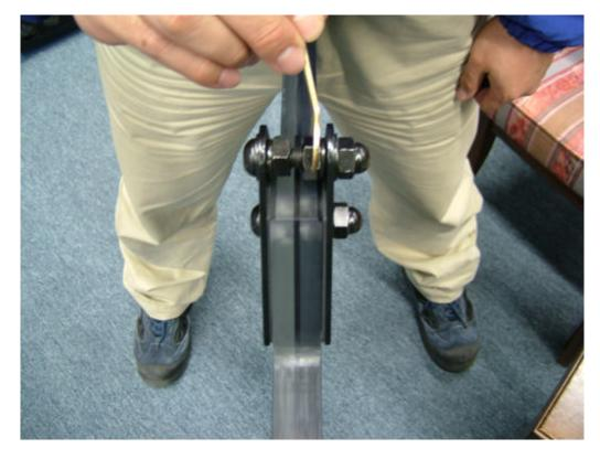
Step 8: Recheck now that all nuts are firmly tightened, be sure to use only the tools provided to ensure no over torque or damage. Be sure that all rubber pads and lock washers are completely compressed.
