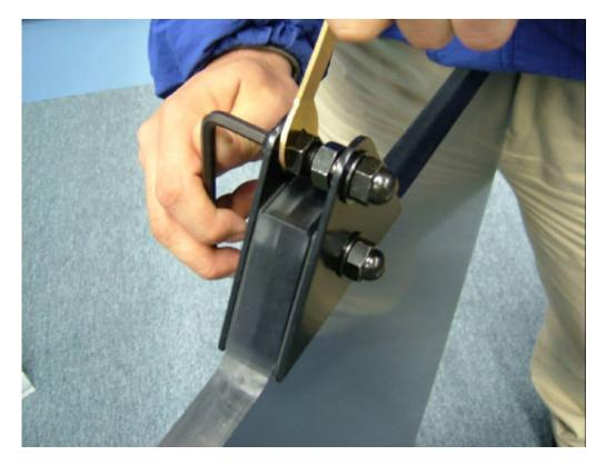
Step 5: Note inner lock washer totally compressed & adjacent nut loose with play.
