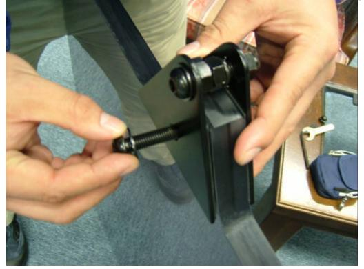
Step 3: Place on washer & firmly tighten nut, completely compressing rubber pads.
