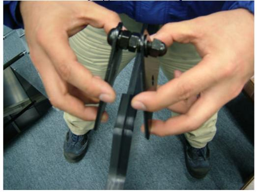
Step 2: Gently insert bottom bolt & washer set and center bracket on screen flange.
