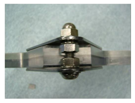
Step 6: Gently tighten cap nut to set bracket the same width as bottom bolt, loosen adjacent inner nut as necessary to make gap exactly the same.
