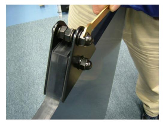
Step 7: Now firmly tighten final inner nut outward, completely compressing lock washer.
