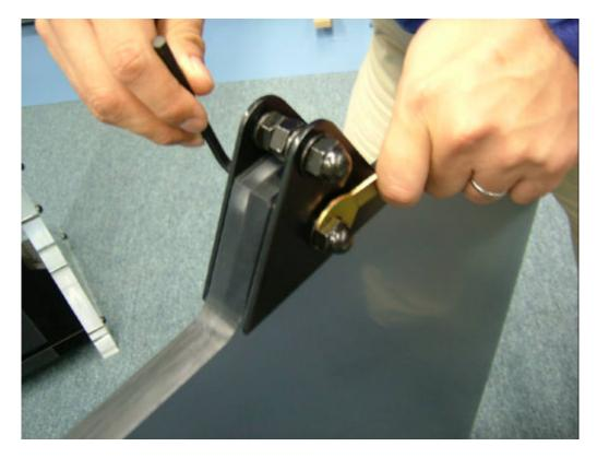
Step 4: Firmly tighten top inner nut nearest bolt head, completely compressing lock washer.
